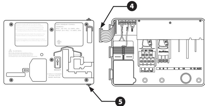
**6** The ESP-SMT Smart Modular controller has a single keyhole slot at the rear top of the cabinet. At the bottom of the cabinet are three circular mounting holes. Mount the controller so that at least one of the bottom holes lines up with a wall stud or other solid surface.
